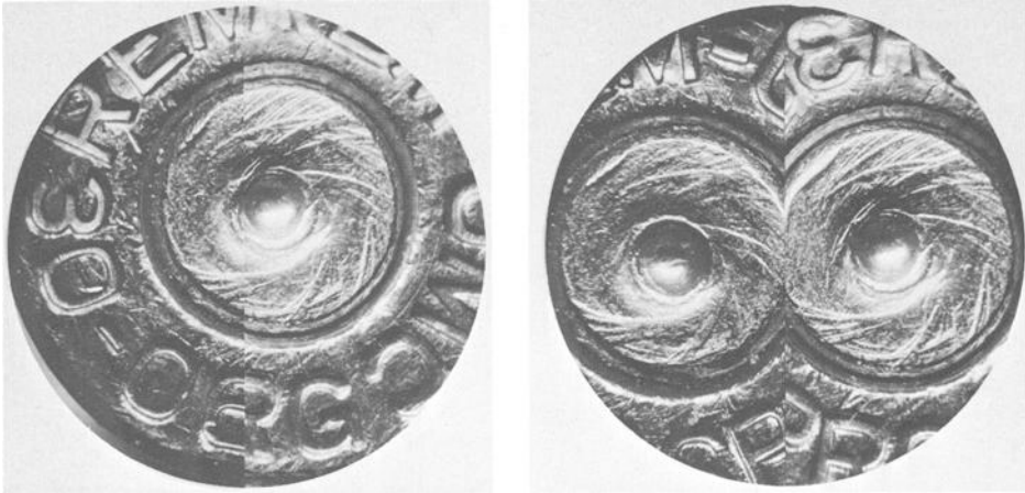
FIG. 3—Comparison photomicrographs demonstrating the identification between cartridge cases recovered near tree to cases from the owner of stolen rifle.
