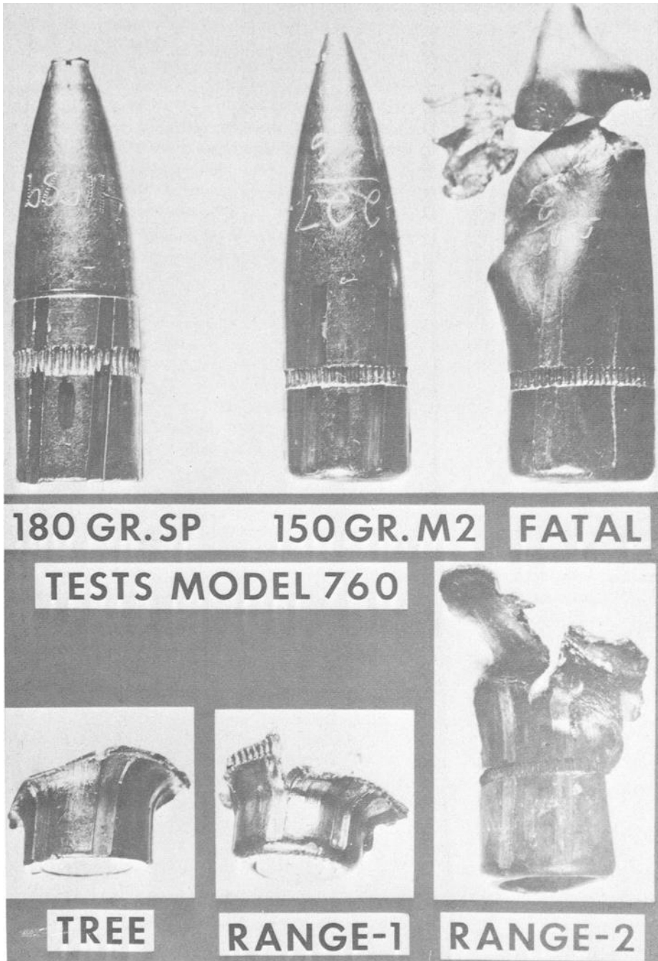
FIG. 1—Bullets used to link the FATAL bullet with the missing murder rifle. The FATAL bullet and the two RANGE bullets are metal jacketed, spitzer, 150 grain M2 ball (U.S. Army) military type. The bullet from the TREE is a 180 grain soft point corresponding to ammunition possessed by the owner of the stolen rifle. The two TESTS were not fired by the murder weapon and are included solely for the purpose of illustrating bullet type and class characteristics of rifling marks.
